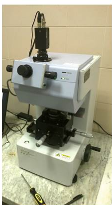
Figure 1. Shimadzu DUH-211S depth-sensing indentation system, with an example of load-unload cycle.
